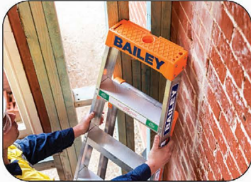
Inside corner leaning
