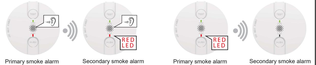
**4 Pairing failure:** The red LED lights on the primary and secondary smoke alarms stay on and the buzzer not making a short beep.
